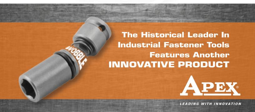
The **Apex WSK Wobble Socket Adapter Kit** can convert any fastener tool with a female square drive (3/8", 1/2", 5/8", 3/4", or 1") and a DIN groove into a Wobble socket. This will enable you to drive fasteners that may have a slight misalignment (up to 10 degrees) between the drive tool axis and the fastener axis. In addition, this will also prove extremely useful in hand-drive operations where clearance may be an issue.
